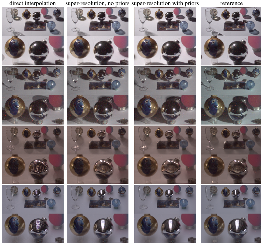
Figure 9: Results of a complex scene with detail zoom-ins for renderings in two point light conditions (upper four rows) and in the Galileo’s Tomb and Uffizi environment maps ( http://debevec.org/Probes/ ). The super-resolution reflectance field is upsampled from 230 to 3547 images, the reference has 14116 images. Our upsampling approach produces superior results compare to linear interpolation. Applying the regularization (second column from the right) further improves shadow boundaries; for real-world illuminations, the non-regularized version is already close in quality. Note that the reference exposes aliasing which the super-resolution images do not show due to sub-pixel blurring during the upsampling steps.
